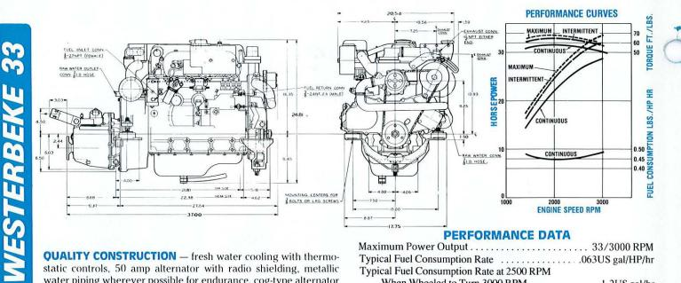
**QUALITY CONSTRUCTION** — fresh water cooling with thermostatic controls, 50 amp alternator with radio shielding, metallic water piping wherever possible for endurance, cog-type alternator belts reduce slippage, glow plug cold weather starting aid, oversized 3" diameter heat exchanger, shut-off function built into throttle control, cast iron head and block for long life.
